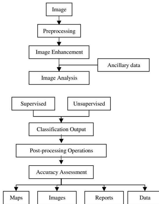
Figure 5 - Fundamental steps in remote sensing image processing .
