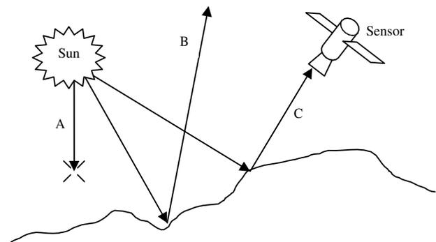
Figure 1 - Sensors measure the amounts of energy reflected from or emitted by the Earth surface targets: Absorbed (A), Scattered (B), and Reflected (C) energy (Adapted from [1]).
